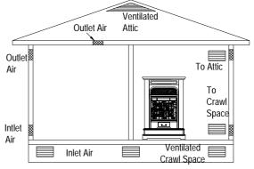
Figure 3-Ventilation Air from Outdoors
